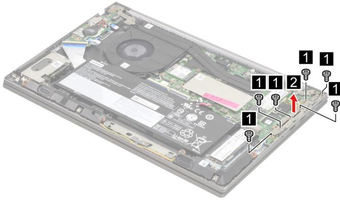
Figure 65. Remove six screws and remove the I/O bracket (left)
