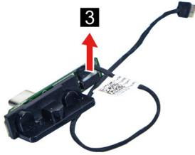
Figure 81. Remove the ear phone Bluetooth board cable
