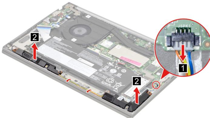
Figure 74. Remove the speakers
