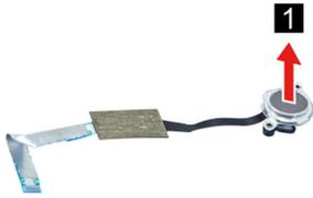
Figure 73. Remove the fingerprint board lens light guide
