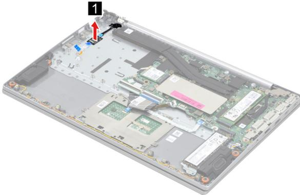
Figure 29. Remove the fingerprint board with cable
