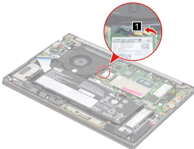
Figure 86. Peel off the mylar
