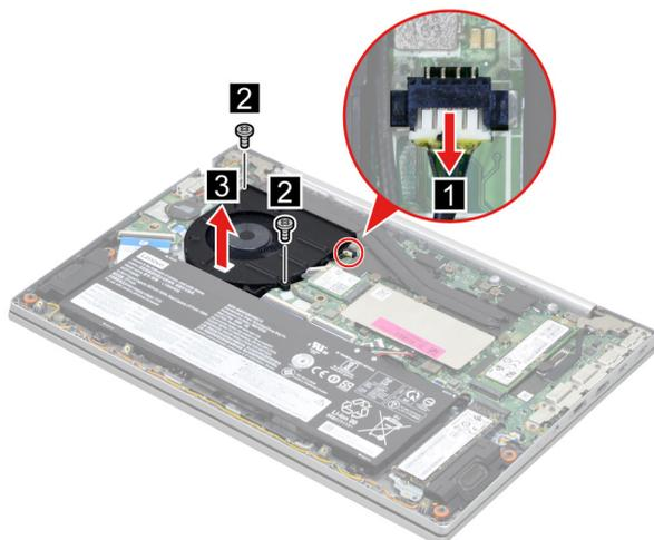
Figure 18. Remove two screws and remove the fan
