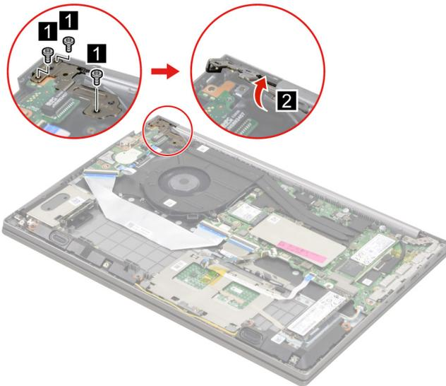
Figure 67. Remove three screws and open the hinge
