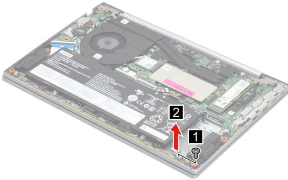
Figure 13. Remove one screw and remove the 2<sup>nd</sup> SSD bracket
