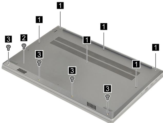
Figure 47. Loosen six screws and remove five screws
