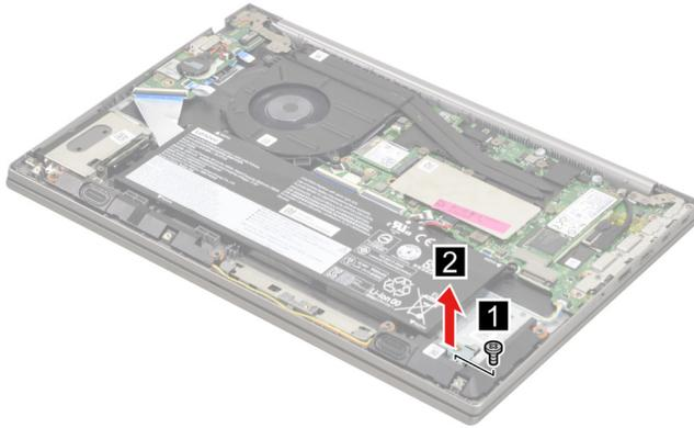
Figure 55. Remove one screw and remove the 2<sup>nd</sup> SSD bracket
