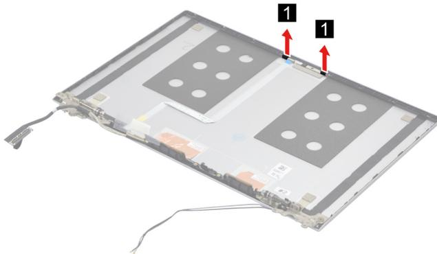
Figure 44. Remove the microphone rubbers
