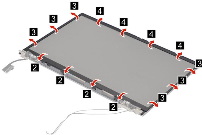
Figure 91. Remove the LCD bezel
