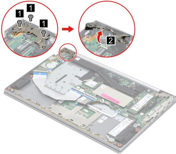
Figure 24. Remove three screws and open the hinge
