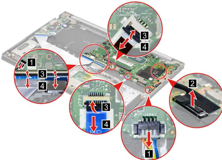
Figure 84. Disconnect cables connected to the system board
